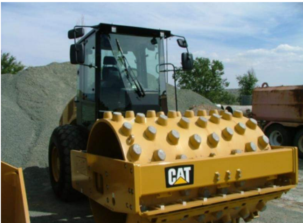
Figure 57: Sheepfoot Roller (Source: the county of Lincoln – Road)
